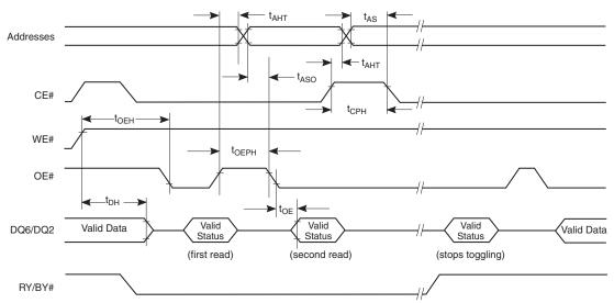
Figure 17.10 Toggle Bit Timings (During Embedded Algorithms)
