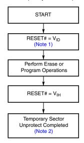
Figure 8.1 Temporary Sector Unprotect Operation
