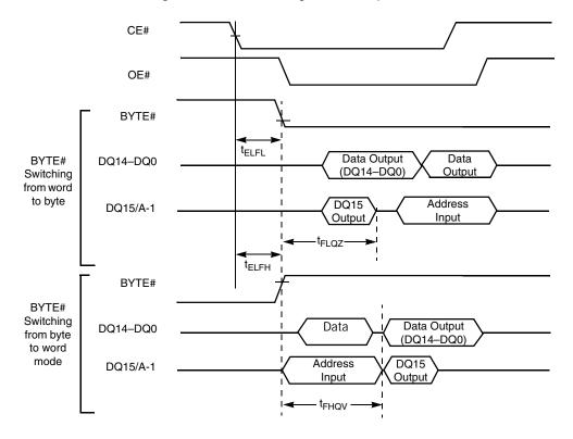
Figure 17.4 BYTE# Timings for Write Operations
