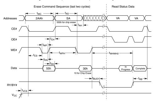
Figure 17.7 Chip/Sector Erase Operation Timings
