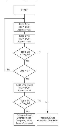
Figure 11.2 Toggle Bit Algorithm
