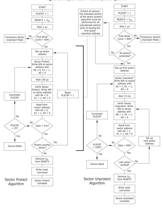
Figure 8.2 In-System Sector Protect/Unprotect Algorithms
