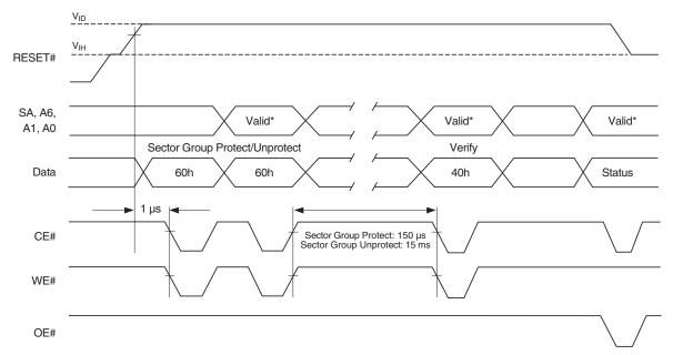
Figure 17.13 Sector/Sector Block Protect and Unprotect Timing Diagram
